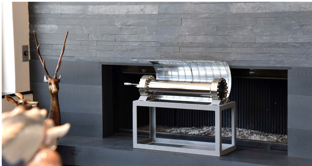
Figure 1. An R20 reactor used as a room heater in Sapporo, winter 2018. With 300 W input, it kept the room about as warm as a conventional 3 kW gas or electric room heater. Such room heaters are common in Japan. The reactor is powered by a 500 W, 100 V laboratory power supply, which is not connected in this photo.
