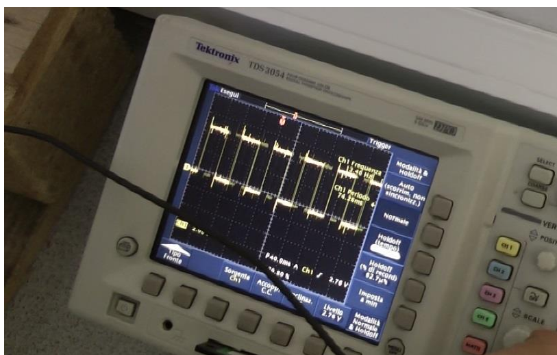
Figure 7 Trace of the digital output signal of the flowmeter during the phase previous to boiling of water in the coil. Note the regular pattern of the pulses in time
